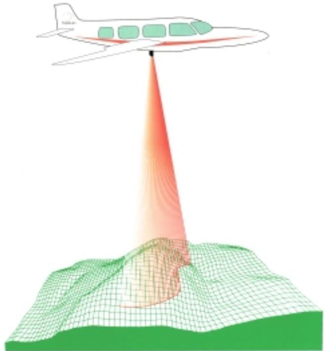
Figure 1: Principle of laser scanning.
