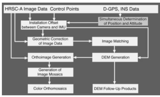
Figure 2: Photogrammetric Processing Line for HRSC-A.
