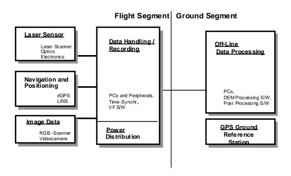
Figure 1: TopoSys system components.
