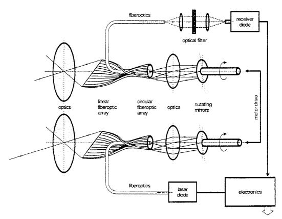
Figure 2: Architecture of the Laser Scanner.
