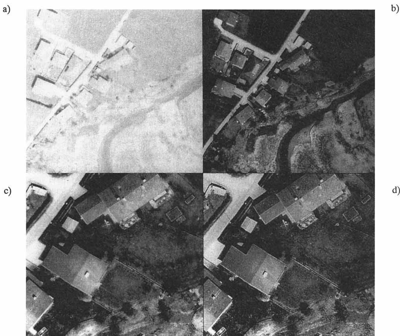
Figure 6a: Portion of original scanner-data in positive representation (histogram see Fig. 5a). Figure 6b: Result of contrast-function F_1 of Fig. 5b applied to Fig. 6a (histogram see Fig. 5a). Figure 6c: Detail of Fig. 6b at full resolution (512 by 512 pixel), local contrast not enhanced. Figure 6d: Result of enhancement applied to original data (with functions F_1 and F_2 of Fig. 5b).
