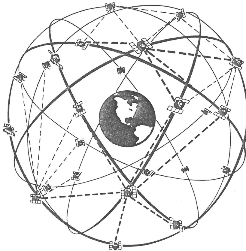
Figure 2: Block IIR satellite configuration with crosslink capability
