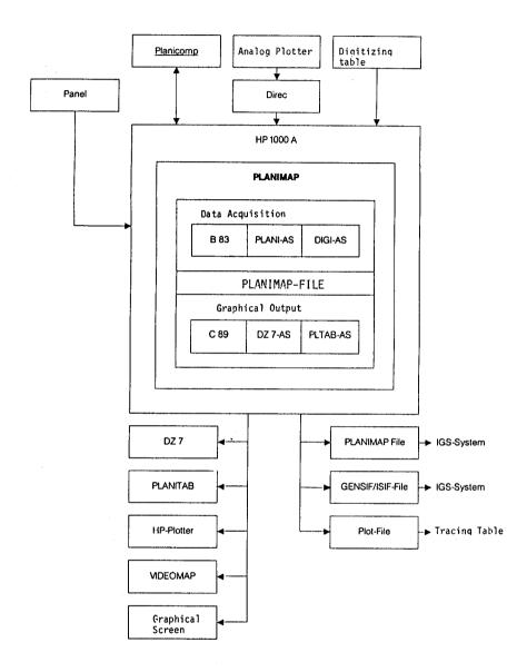
Fig. 1: Schematic overview of the PLANIMAP digital mapping system
