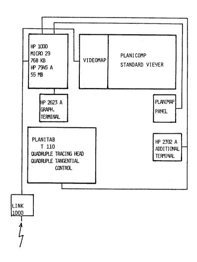
Fig. 2: Photogrammetric plotting centre with Planicomp
