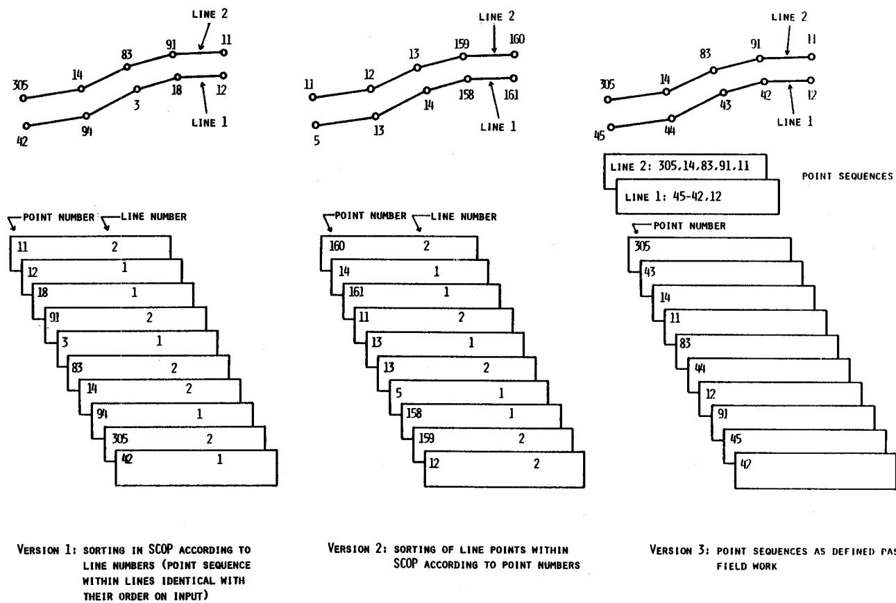
Fig. 5: Versions of collecting line information (terrestrial data acquisition)
