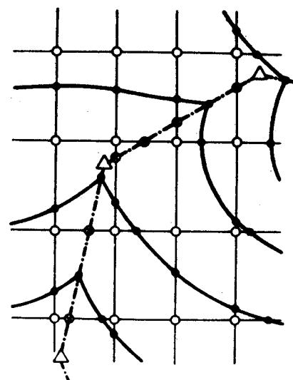
Fig. 2: Contour lines interpolated in a DHM with breaklines
