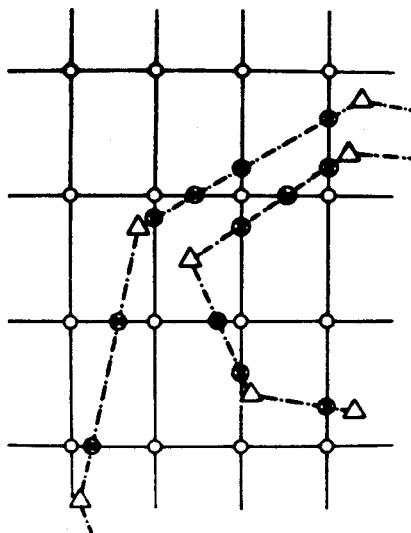
Fig. 1: DHM - rectangular grid with intermeshed breaklines
