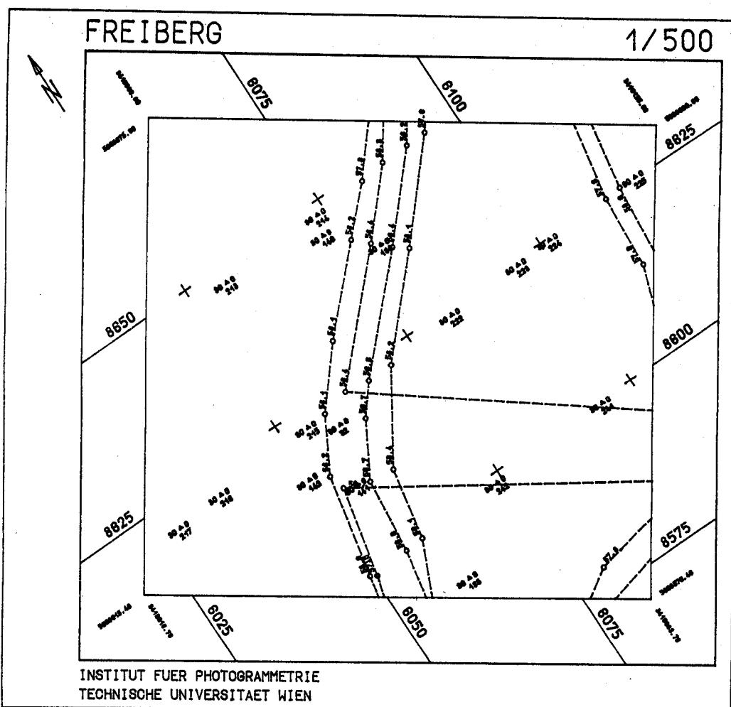
Fig. 8: Data plot of single points (=RANDOM) and of breakline points (=BREAKLINES); other parameters to the directive DRAW: PSYMB=3: triangle, PSYMB=7: circle, LSYMB=2: broken line, Z: with Z-coordinates, ADDR: with UPDATE-addresses.
