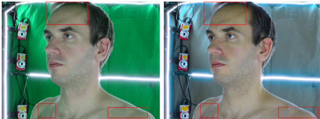
Figure 2.3: Example of colour correction automatically generated, highlights some areas where the green reflection can be seen on the user skin.
