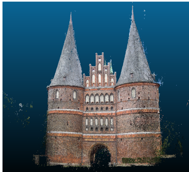
Figure 4: FBM-based automatic network orientation: (a) Network geometry of 43-station, 240,000-point network, (b) 3D model comprising 50 million points from SGM-based dense matching.
