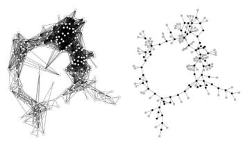
Figure 2: Reducing the full match graph (left) to a skeletal set (right) greatly reduces the number of image pairs that need to be matched, while nevertheless preserving an acceptable camera network for reconstruction. Figure courtesy of N. Snavely.
