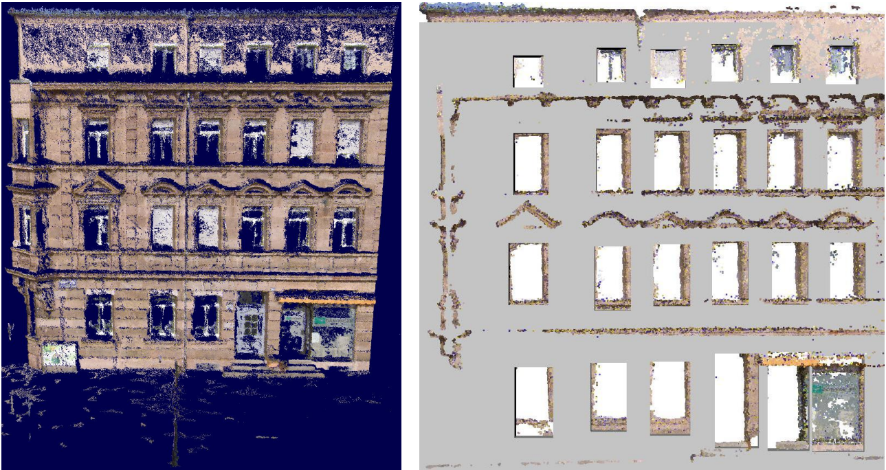
Figure 5: Dense 3D point cloud (left) and windows as well as doors as holes in the façade plane (right).
