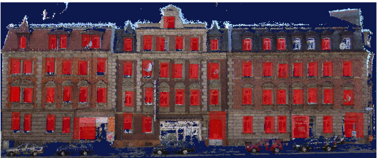
Figure 6: Dense point cloud of several façades with windows and doors marked by red boxes.
