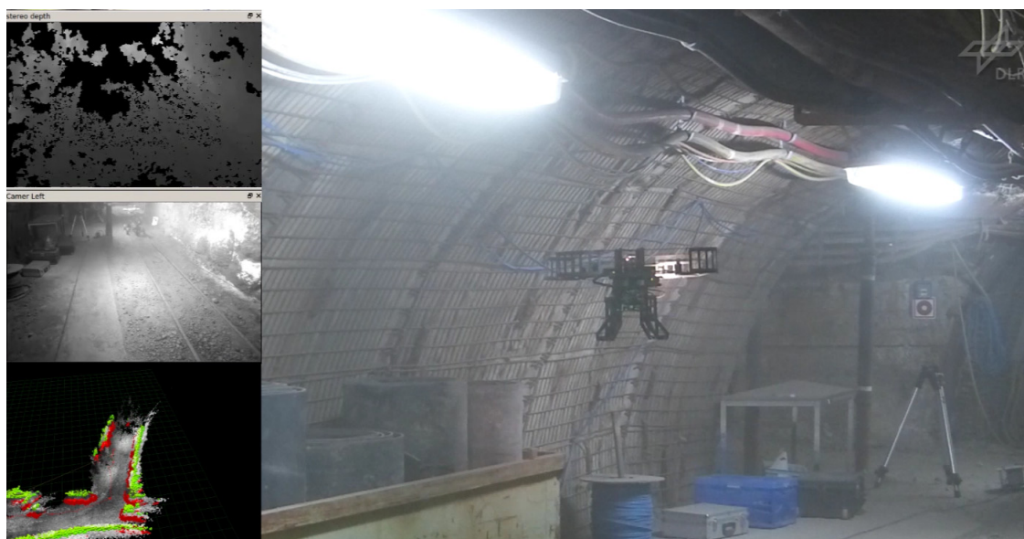
Figure 7: Autonomous flight of the DLR Pelican quadcopter in a coal mine.
