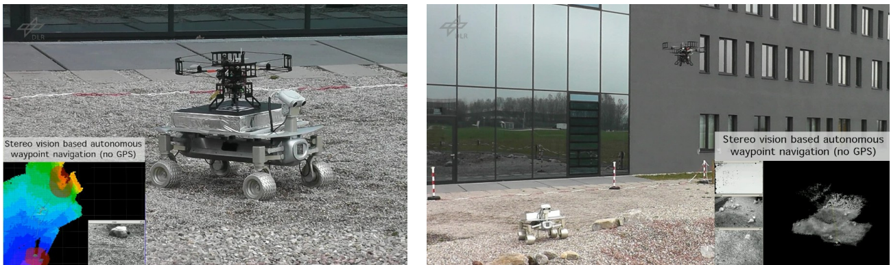
Figure 9: Rover as carrier for a quadcopter. Both systems are operated by autonomous waypoint navigation.
