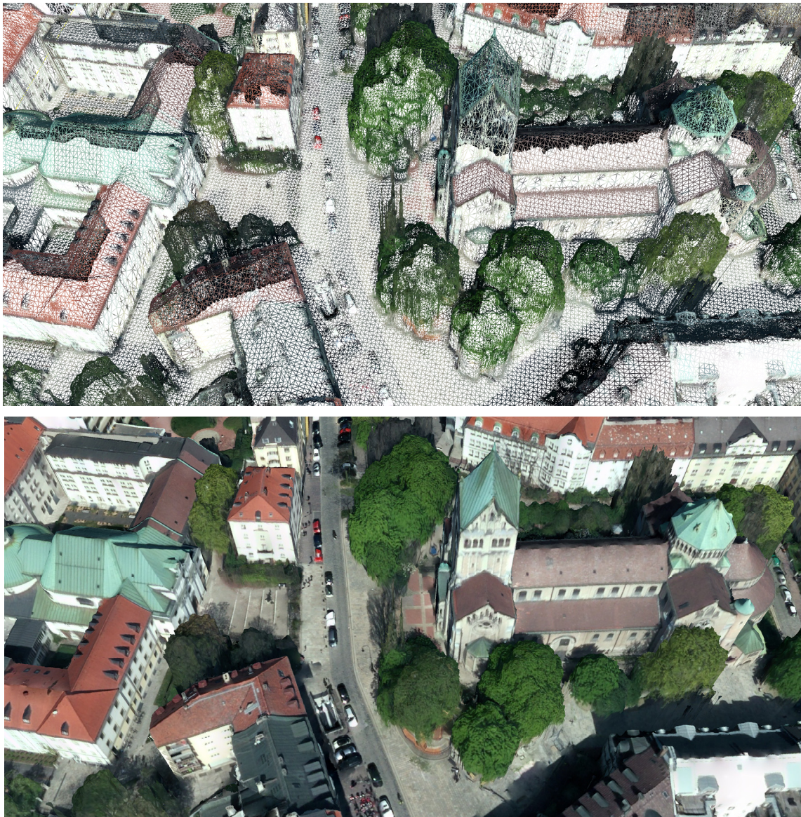
Fig. 4. Texture mapping for triangulated DSM raster, visualisation of vertices (top) and faces (bottom).
