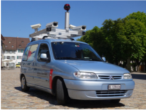
Fig. 8: Platform and sensor configuration of the IVGI mobile mapping system.
