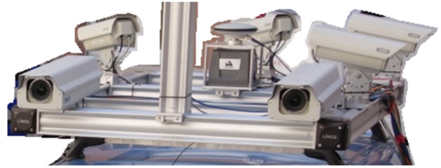
Fig. 8: Platform and sensor configuration of the IVGI mobile mapping system.
