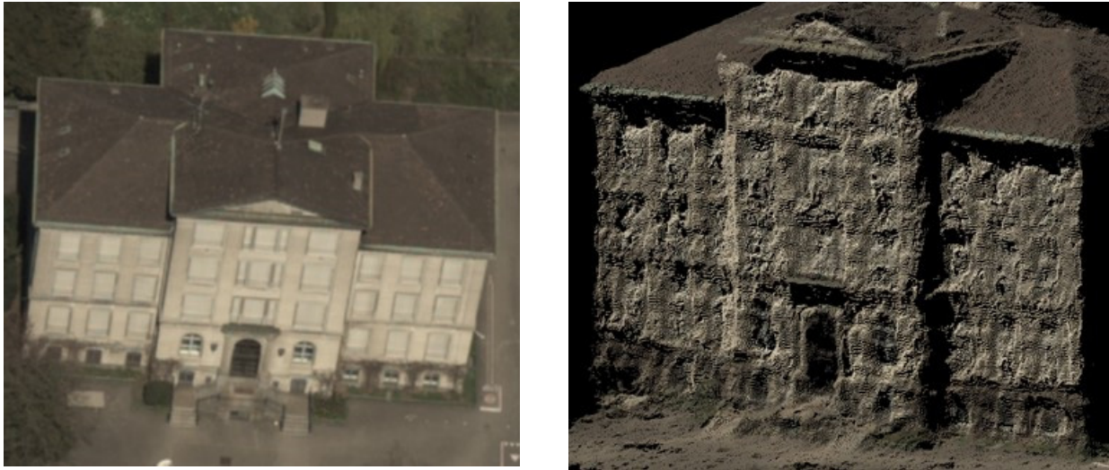
Fig. 5: Façade image in oblique view (left) and corresponding 3D point cloud (right) from dense image matching.
