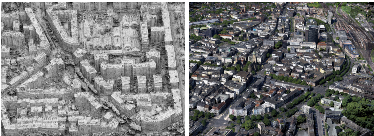
Figure 4: Example of dense point clouds from oblique datasets. Shaded view produced with MicMac from a MIDAS dataset (left) and colour cloud obtained using SURE on a PentaCam IGI dataset (right).
