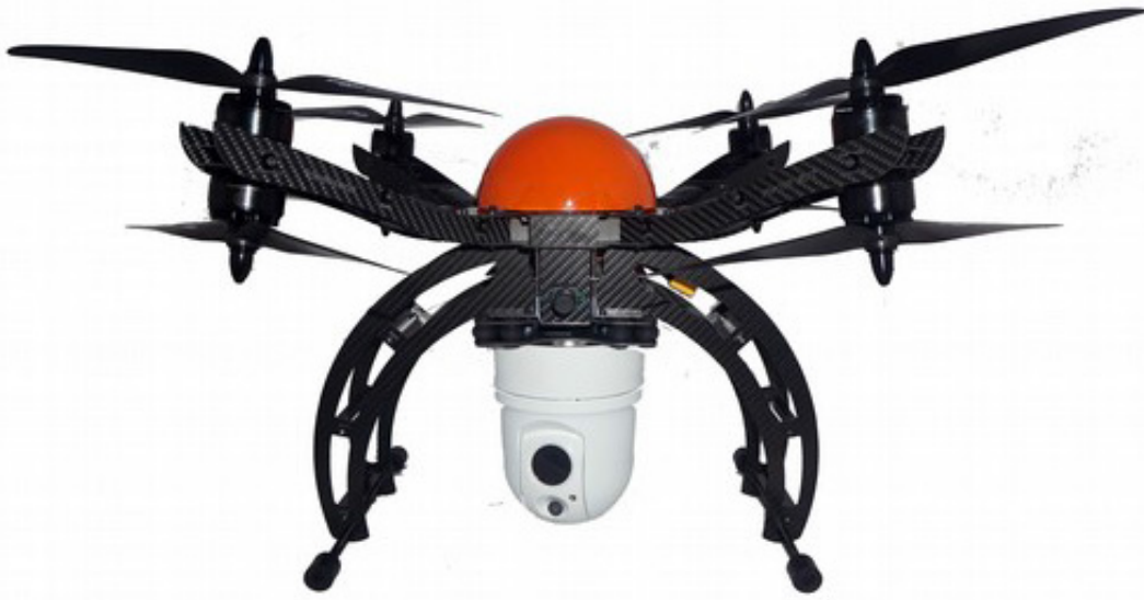
Figure 4: G47S – surveillance rotary wing UAV.
