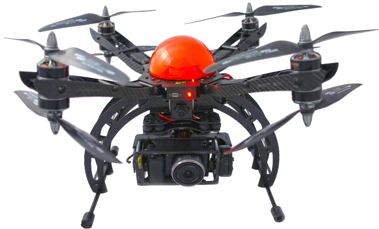
Figure 3: G47-X8 – rotary wing UAV, co-axial octocopter.
