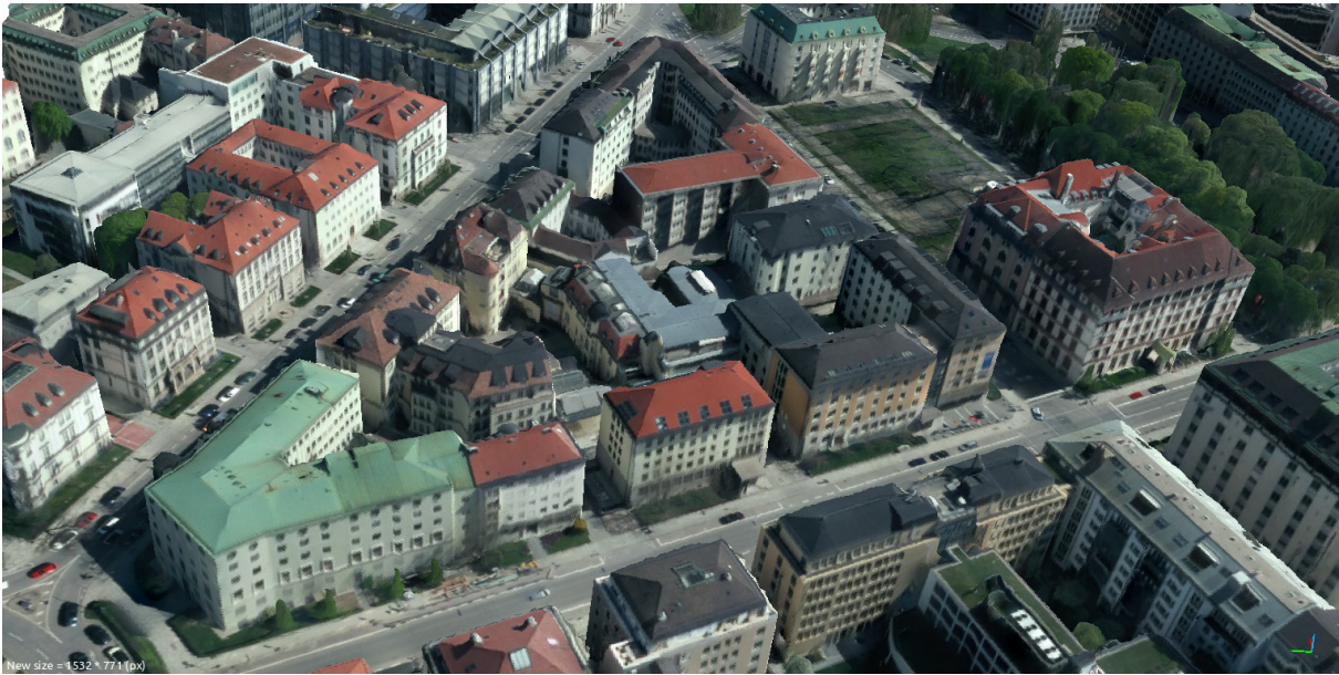
Figure 5: Textured mesh automatically generated from the Munich EuroSDR data set (Haala, 2014) (Nadir Configuration, GSD 10 cm, Overlap: 80% in strip, 80% across strip).
