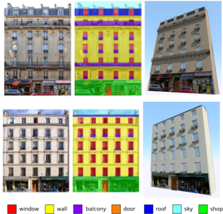
Figure 9: Some modeling results on the ECP dataset. Left: original image. Middle: semantically segmented facade. Right: procedural building model.
