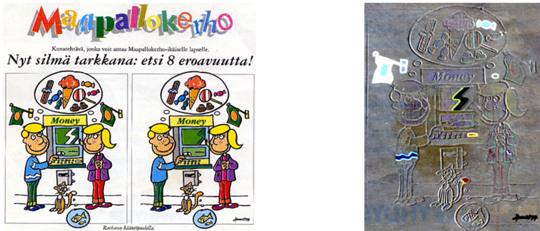
Figure 3: Change detection problem for kids. Find 8 differences from the left image pair. Difference image produced on the right. In image differencing, the co-registered images are simply subtracted from each other. The differences are easily detectable. Courtesy to Maapalokerho.
