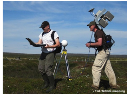
Figure 1: The backpack MLS system of FGI.
