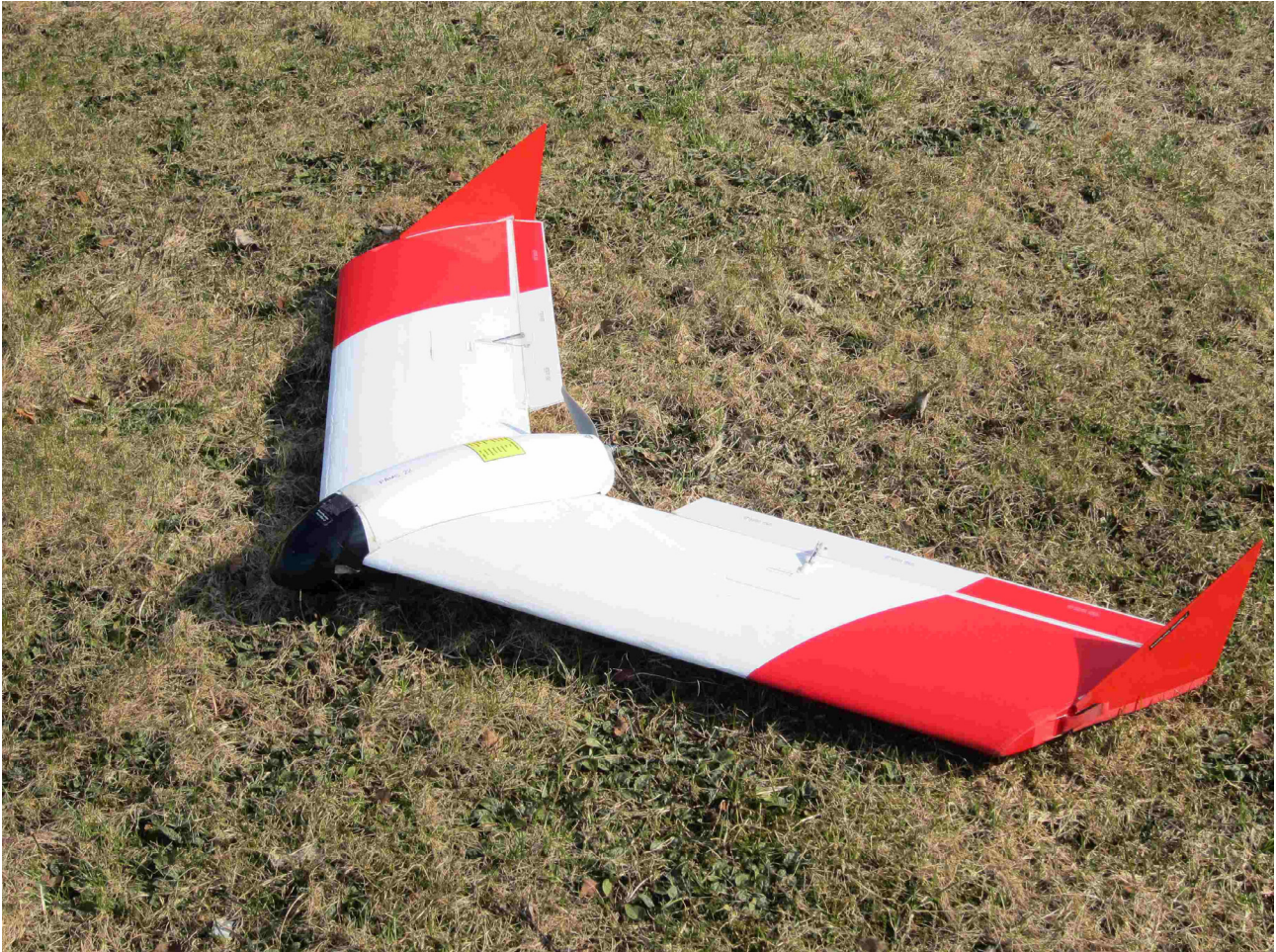
Figure 2: SmartOneC, RPAS, 1.2 kg MTOW, 120 cm wingspan.
