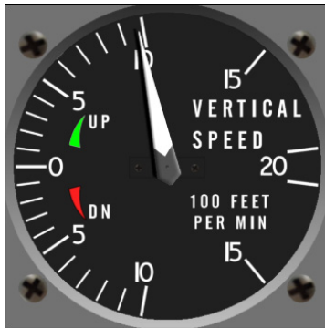
Figure 5: Vertical Speed Indicator.
