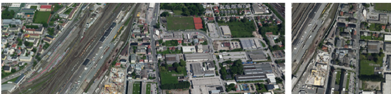
Figure 4: Forward wing image (composite of twin cone) and part of nadir image (right).
