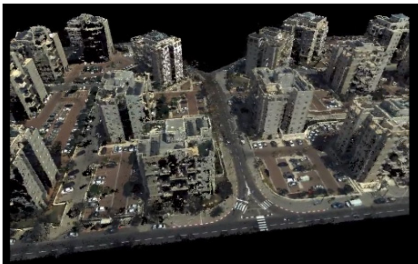
Figure 6: Point cloud generated using SGM.
