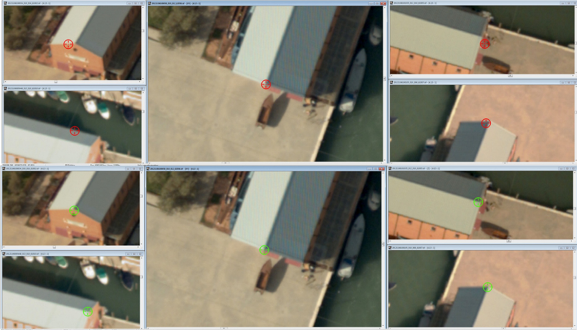
Figure 14: Leica RCD30 oblique imagery before and after tridicon ® APM Trio blockmatching and triangulation.
