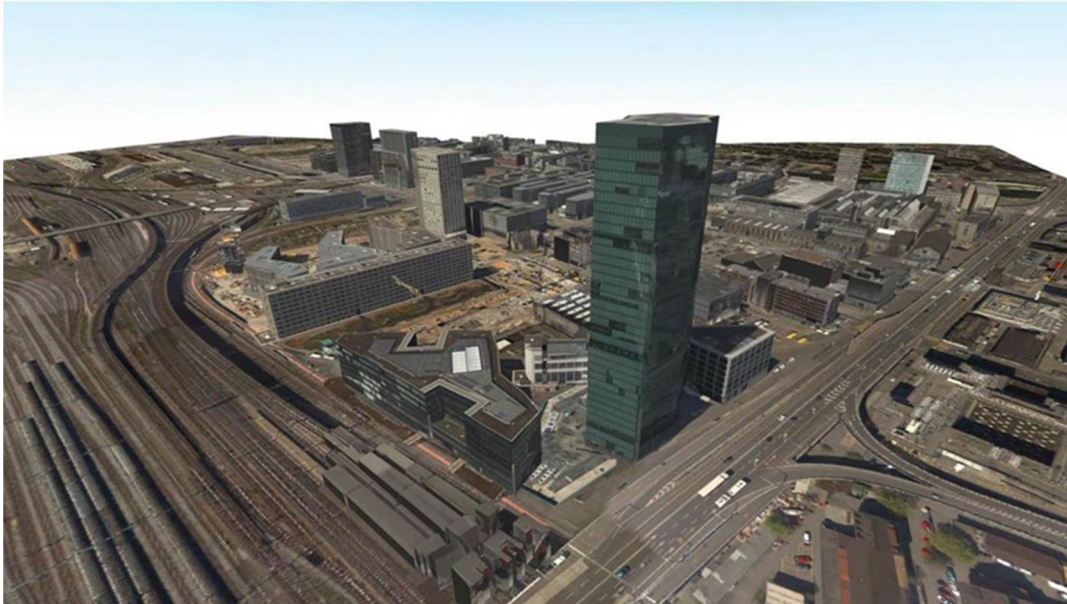
Figure 16: Zuerich West 3D city model with Prime Tower automatically generated from Leica RCD30 oblique data without any other information.
