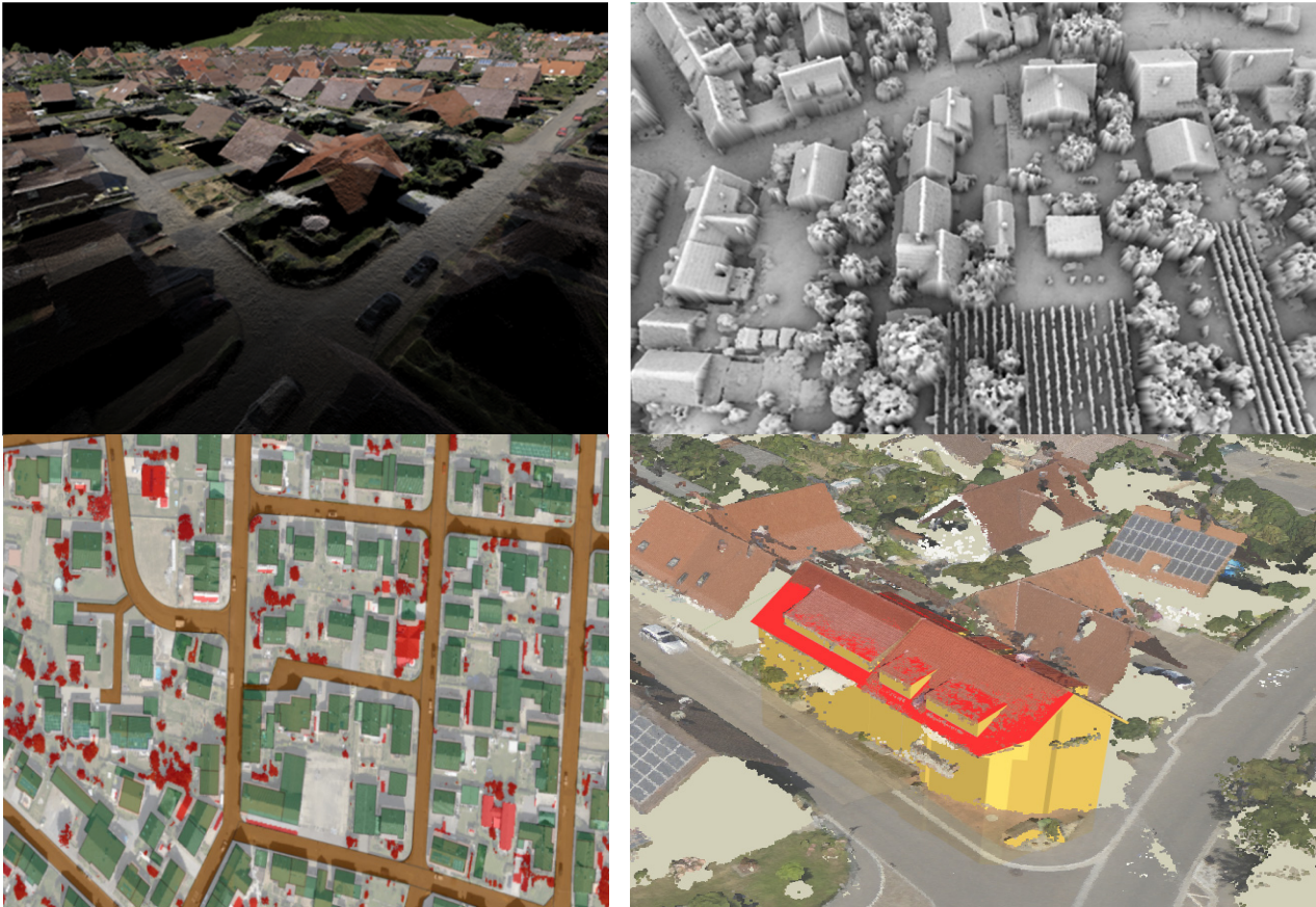
Figure 2: Hessigheim colored point clouds (upper left), grey-shaded point cloud (upper right), unregistered buildings (lower left), and manually reconstructed 3D CSG building model (lower right).
