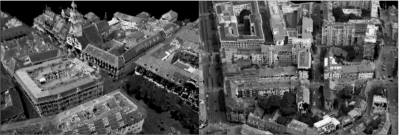
Figure 2: Results for the matching and triangulation for a single stereo model (Microsoft Ultracam, 8cm GSD).
