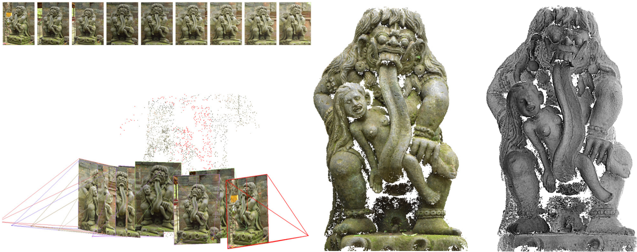
Figure 13: Dense image matching for cultural heritage applications. From left to right: images, image orientation by VisualSFM (cameras and sparse point cloud), dense point cloud from SURE, shaded point cloud from SURE.
