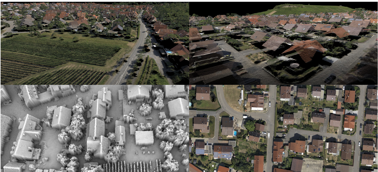
Figure 9: Aerial image dataset with 5cm GSD acquired from a gyrocopter. Upper images: point cloud, lower left: shaded point cloud, lower right: true orthophoto automatically derived from the point cloud.
