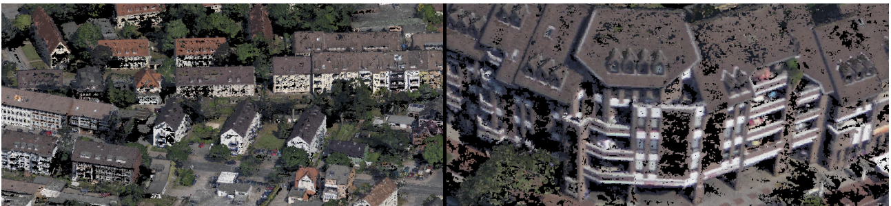
Figure 10: Point clouds from a IGI Quattro DigiCAM Oblique with four cameras looking in a 45° angle.
