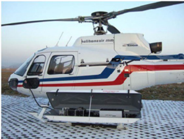
Figure 13, 14: Certified Pod for AS-350 (FAA, CAA, EASA); R44 with LiteMapper system.
