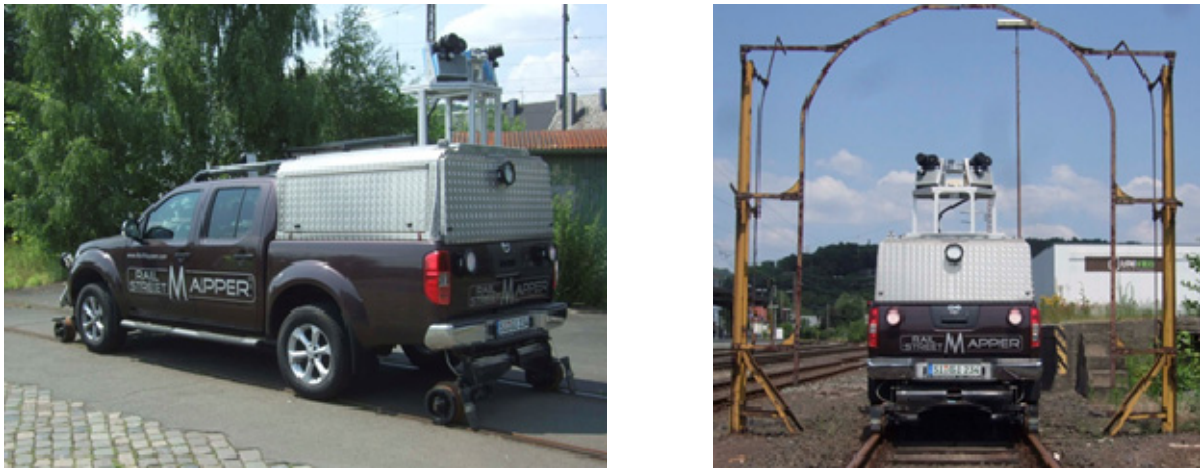
Figure 17, 18: Rail- & StreetMapper system on a two-way car with two Zoller+Fröhlich lasers.
