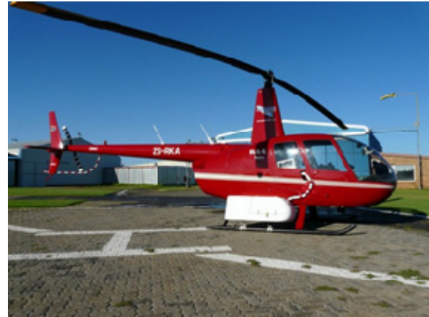
Figure 13, 14: Certified Pod for AS-350 (FAA, CAA, EASA); R44 with LiteMapper system.
