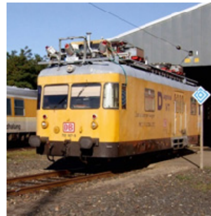
Figure 15, 16: RailMapper system with two laser scanners on a TVT-700 (red) and with three laser scanners on a DiagnoseVT (yellow).
