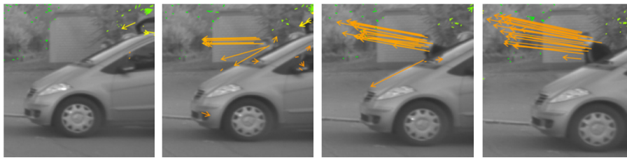
Figure 4: Image sequence with 6D-Vision result. The shown arrows point to the predicted position in 0.5s.
