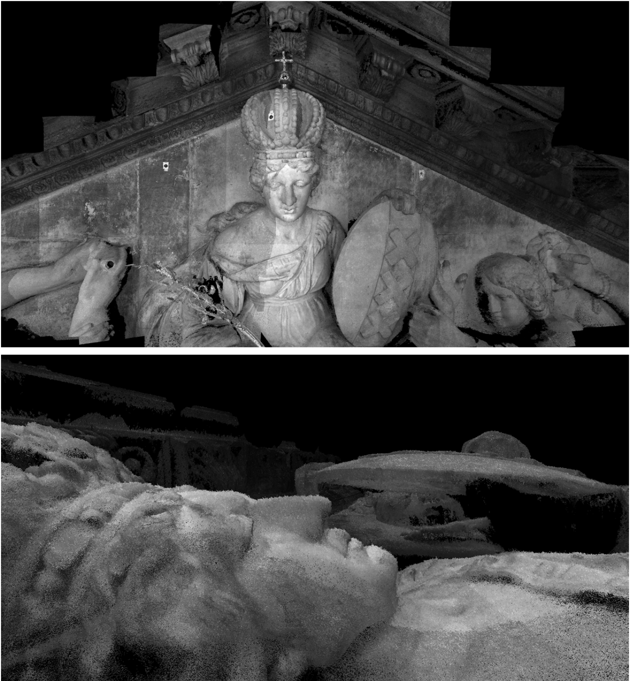
Figure 10: Extracts from the Amsterdam dataset. 58 Mio. points derived directly from the 5 Megapixel bundle camera for about 66 stations. The orientations were derived using Structure from Motion methods. (a) front view onto the point cloud, (b) tilted view.
