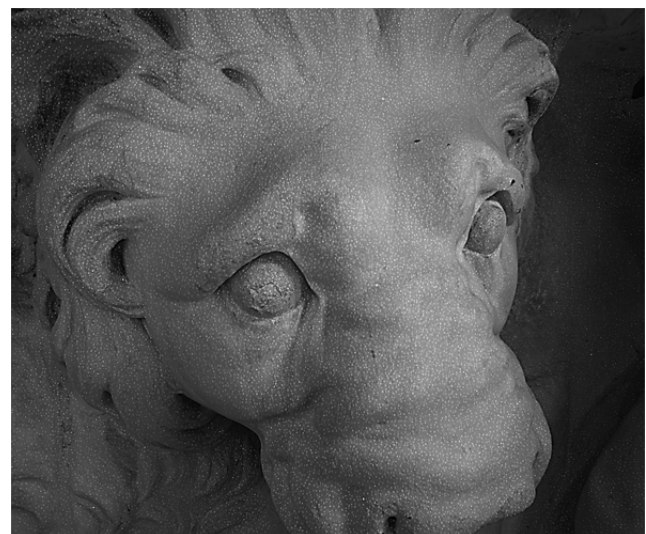
Figure 7: Image taken by one of the matching cameras. The white speckles covering the lion head's surface are produced by the Kinect's IR laser projector and are not visible to the bundle camera. The image has been slightly enhanced to make the pattern easier to see for the reader.
