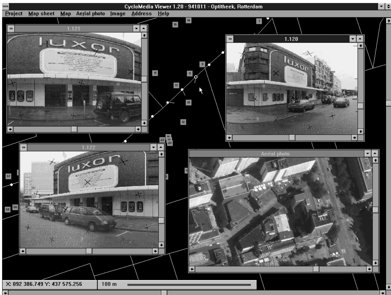
Figure 5: Image Viewing System screen with three panoramic images and an aerial photo, looking towards a selected address
