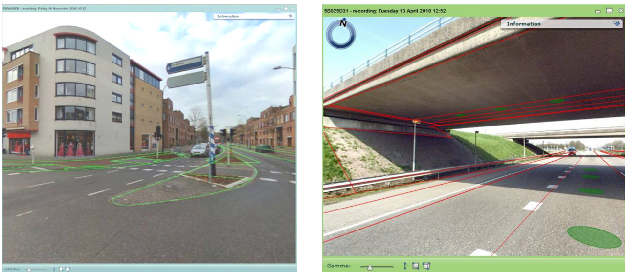
Figure 8: Projection of 2D and 3D vector data on panoramic images
