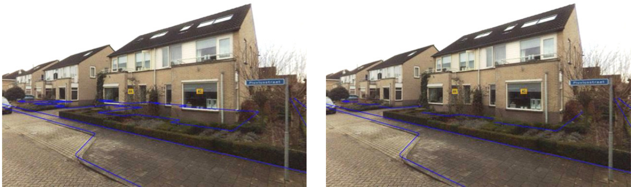
Figure 13: Removal of occluded lines from an overlaid 2D map
