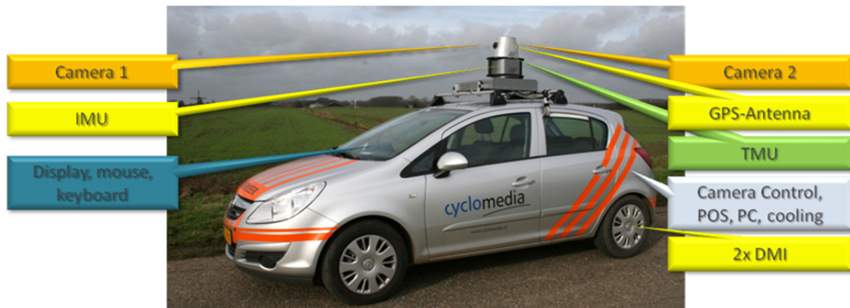
Fig. 7: Major components of the Recording System
