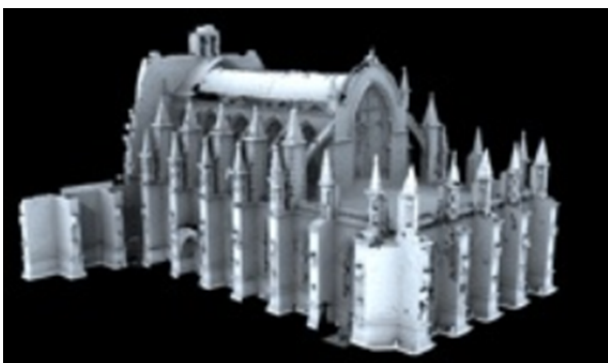
Image Five: 3D Mesh Model of Chapel exterior – metal shed roof virtually removed
