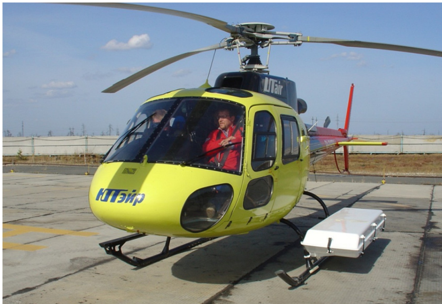
Figure 3: LiteMapper Multi Sensor Platform operated on an AS 350 helicopter in the Russian Federation.
