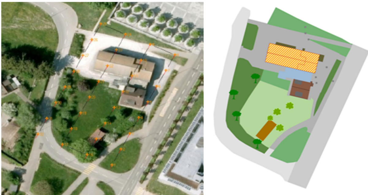
Figure 4: Left: Flight planning of the UAV flight over the test area Campus Science City ETH Zurich (Hoenggerberg). Right: Generated map out of the UAV images.
