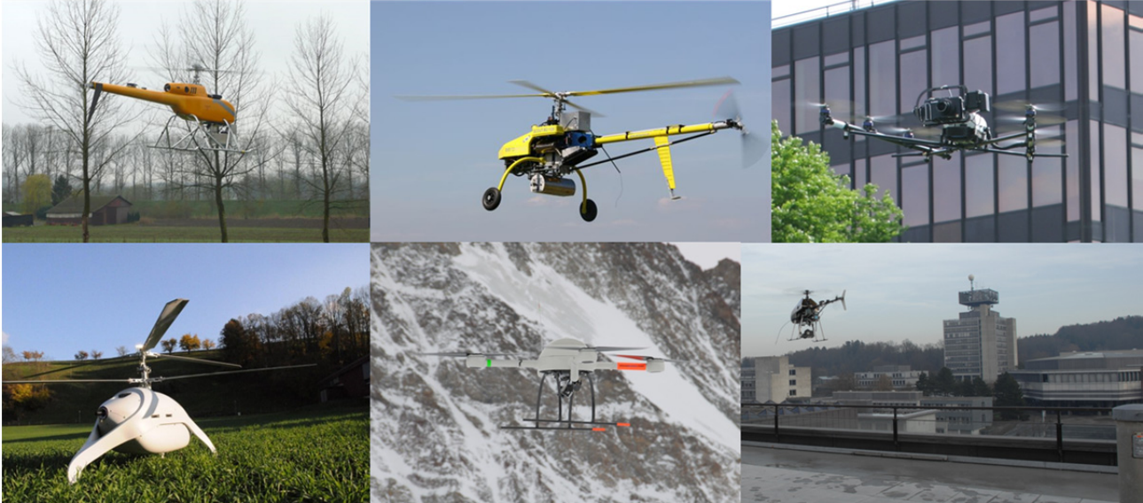
Figure 2: Selection of UAV systems used at the Institute of Geodesy and Photogrammetry (ETH Zurich) for mapping projects.
