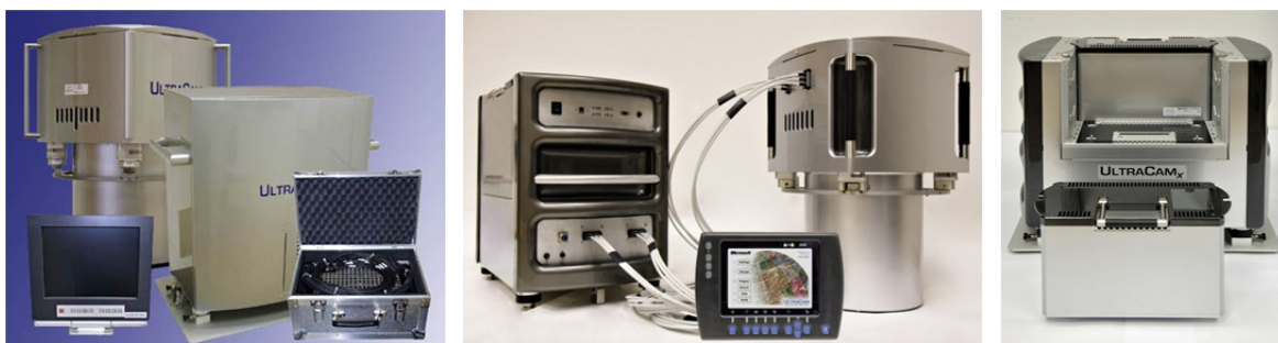
Figure 3: UltraCam D (left), UltraCam X (Xp) complete equipment (middle) and UCX data unit (right).
