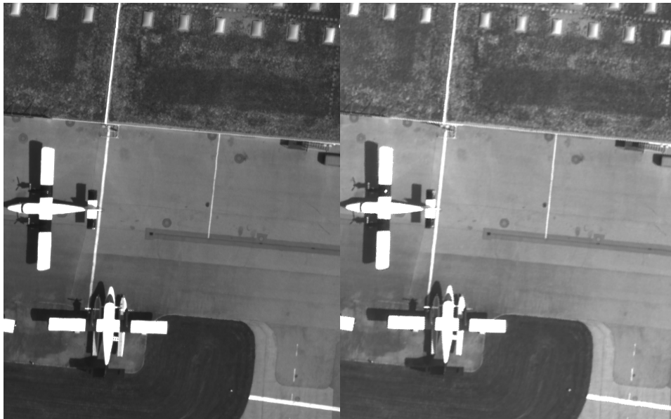
Fig 6: Panchromatic images acquired in standard mode (10cm GSD @ 1000m AGL) and HiRES mode (10cm GSD @ 2000m AGL)
