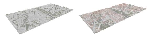
Fig. 9: A virtual 3D model of the center of Graz, Austria is generated by taking into account the semantic classification and the available 3D height information. The model on the left presents the raw DTM and the class "tree", each tree being modeled as an individual point cloud. The right model includes the extracted building blocks, assigning to each block a mean color and height.
