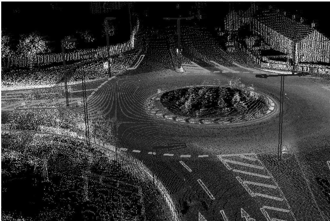
Fig. 9: StreetMapper point cloud data with extracted CAD data.
