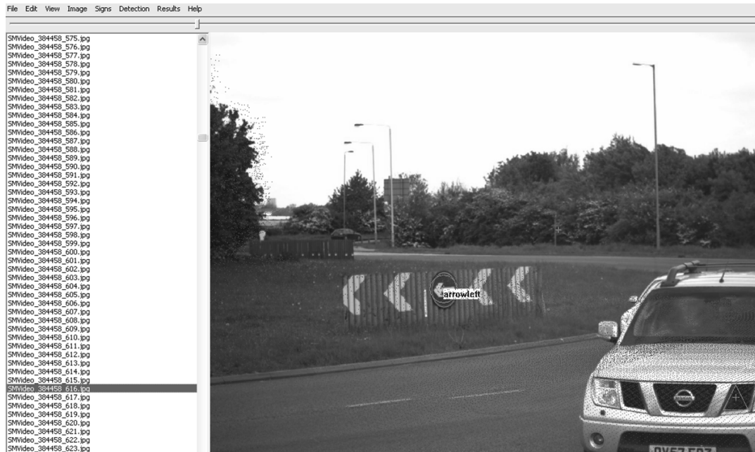
Fig. 10: StreetMapper feature extraction showing two results, with only one validated as correct.
