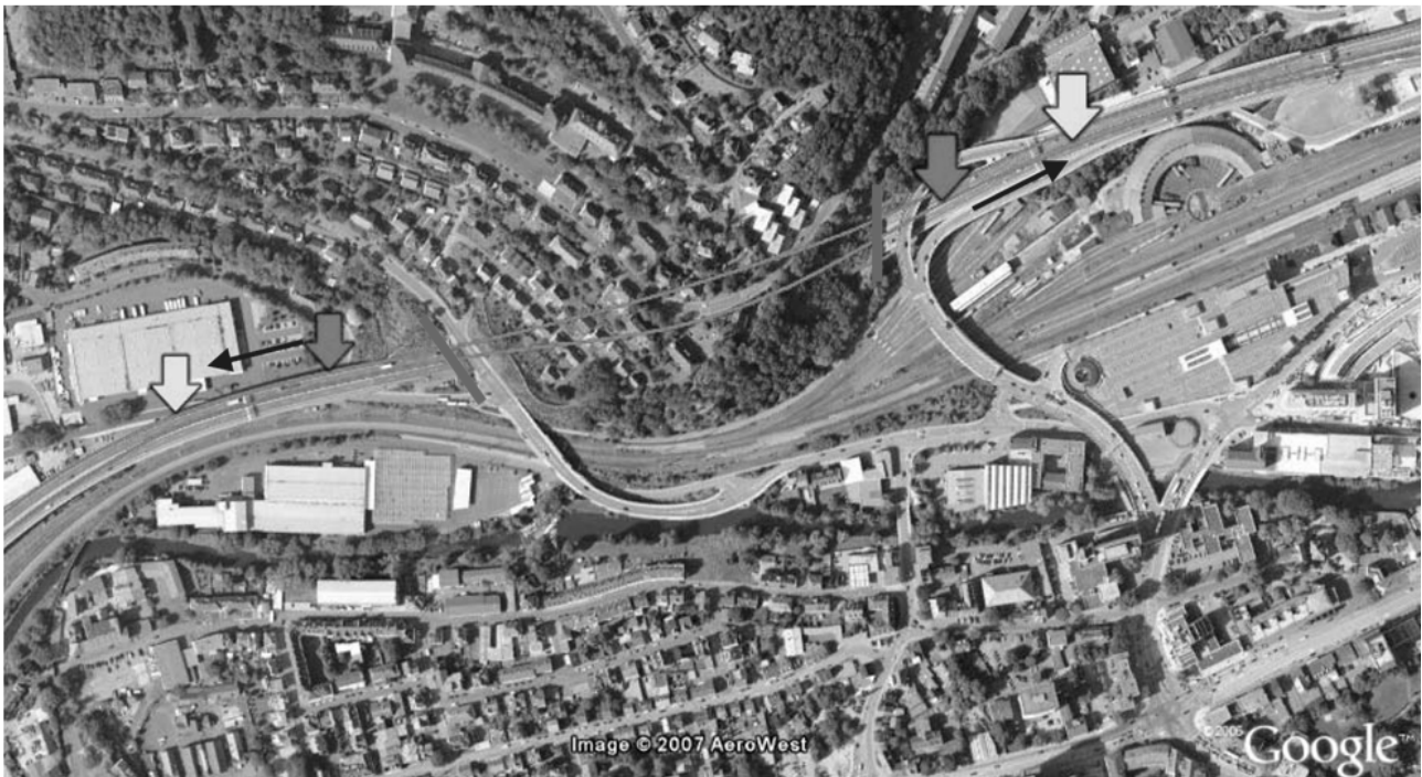
Fig. 5: Plan view of the test area showing tunnel exit lines and arrows showing points where 8 satellites are visible with (dark arrow) and without (light arrow) Direct Inertial Aiding.
