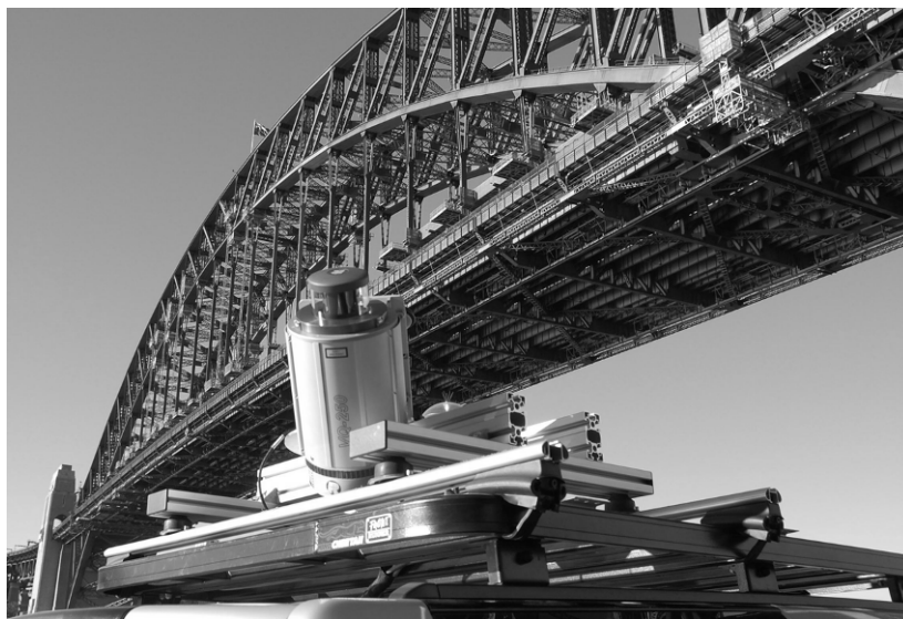
Fig. 8: StreetMapper Portable system in action.
