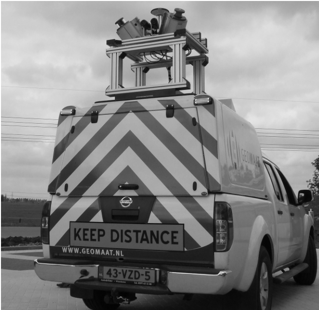
Fig. 6: Lift mount with extra height bars.
