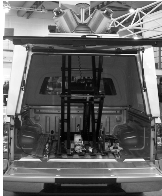
Fig. 7: Hydraulic lift inside vehicle.
