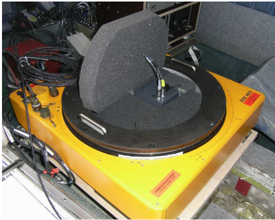
Fig. 8: DigiTHERM with thermal insulation mounted in a GSM3000 mount.
