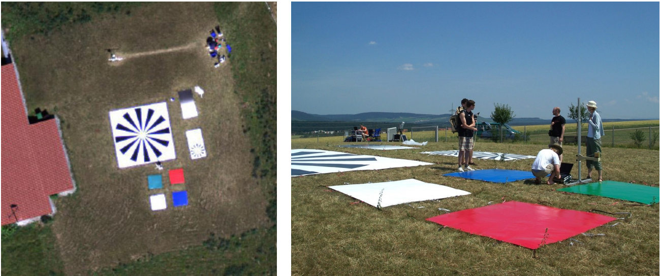
Fig. 3: Vaihingen/Enz radiometric test field from the air (left) and ground team members performing spectrometer measurements parallel to sensor flights (right). Note that airborne and terrestrial image were taken on two different flight days, i.e. the four colour targets were arranged in different order.
