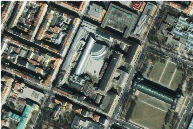
Fig. 2: Satellite image of Munich, Test area TUM, GSD: approx. 1m x 1m, IKONOS
