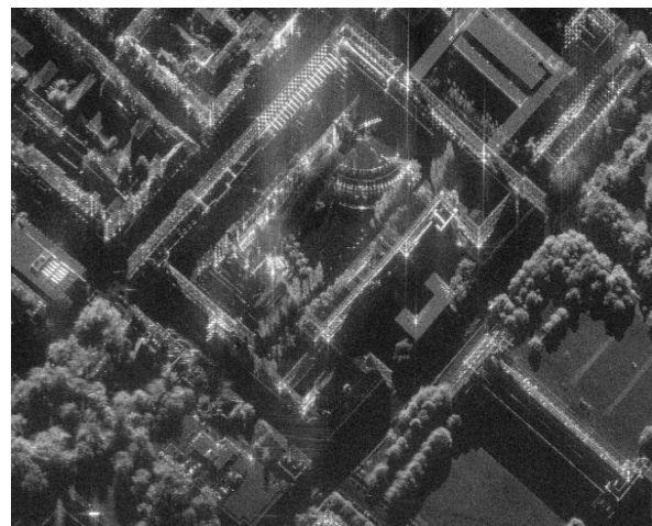
Fig. 5: SAR image of Munich, Test area TUM, GSD: approx. 0.2 m x 0.2 m, MEMPHIS, FGAN-FHR
