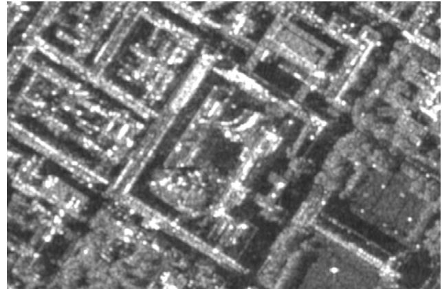
Fig. 3: SAR image of Munich, Test area TUM, Resolution: 2.0 m x 3.0 m (Range x Azimuth), GSD: approx. 0.7m x 0.7 m, E-SAR, DLR-HR
