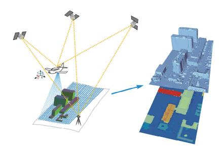
Figure 1: Aerial laser scanning from the eLearning program "Remote Sensing" from the IPF Karlsruhe (see also E. Steinle, Dissertations Karlsruhe, 2005)
