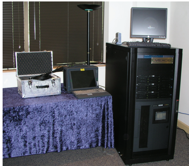
Figure 8: The UltraMap Server satisfies the new need for managing, processing, cataloging, archiving and protecting digital image harvests from the UltraCam-D. An unlimited number of images can be managed in such a tape archive. A subset of perhaps a few 100,000 is kept near-line, and current images are online. Access is via a web browser.
