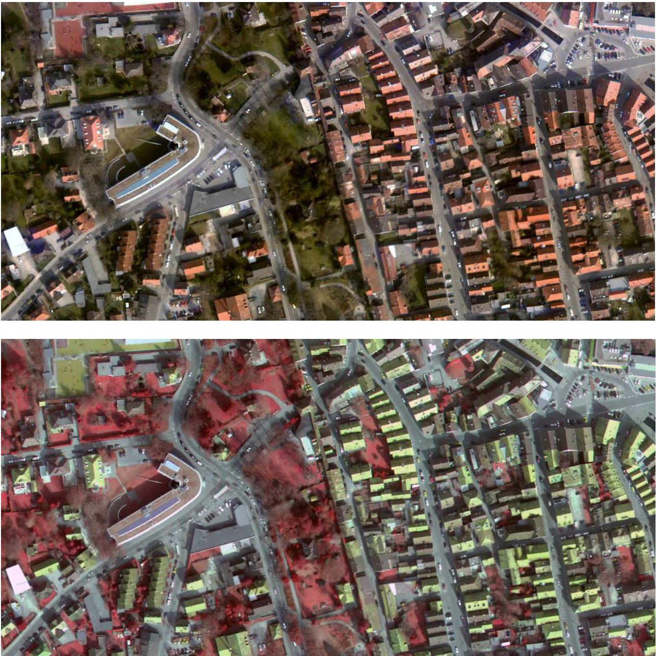
Figure 1: True-ortho images rectified with help of a raster DEM.
