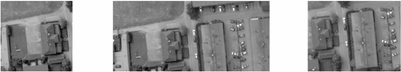
Figure 7: Illustrating the stitching of separate image segments. At the left and right are segments from two component images to be stitched, showing their overlapping region of about 250 pixels. The center shows the seam after stitching is complete. This is taken from Figure 6.
