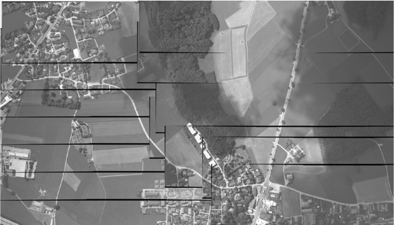
Figure 5: Block of UltraCam imagery in two strips of an area near Salzburg (Austria). The ground sampling distance GSD is 9 cm. Using the 100 mm lens, the flying height is 1000 meters. The image format in this prototype data set is at 11,500 x 2,700 pixels. The black lines serve to mark the individual images.
