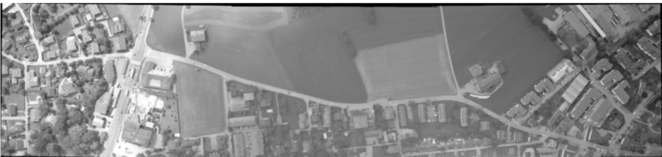
Figure 6: A single image from the prototype camera at 11,500 x 2,700 pixels, taken from the block in Figure 5, composed from 3 separate CCD recordings used in 2 optical cones.
