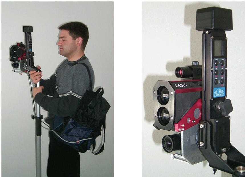
Figure 2: NEXUS georeferencing device
