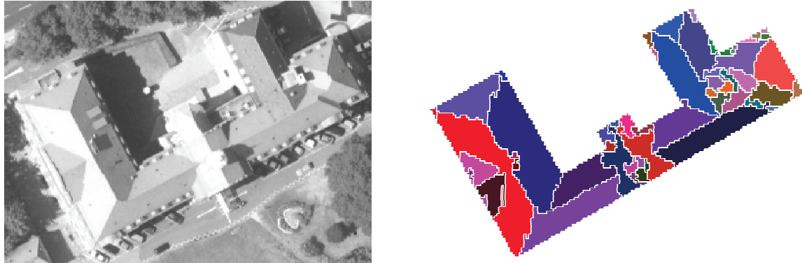
Figure 6. Left: aerial image of a building with complex roof. Right: regions obtained from a planar DSM segmentation.
