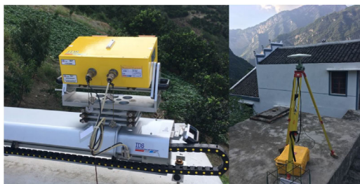
Figure 1: Ground-based SAR and GNSS measurement at Three Gorges Dam
