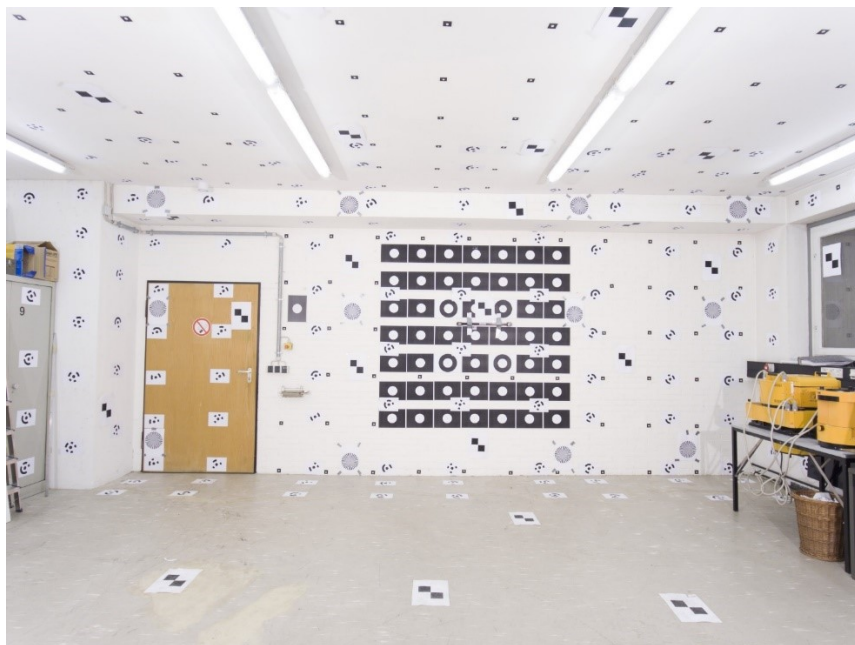
Figure 7: 3D test site for geometrical camera calibration in the ifp measurement lab. In addition to the coded target, several Siemens stars are distributed in the test field to estimate the physical resolution of the sensor system.
