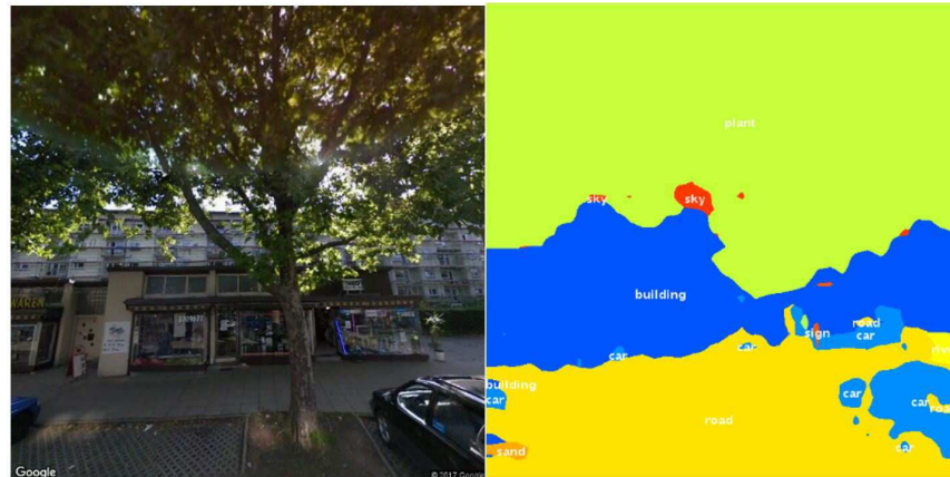
Figure 2: Semantic segmentation of SV images to discard unsuitable candidates. This example would be discarded due to large occlusions by vegetation.
