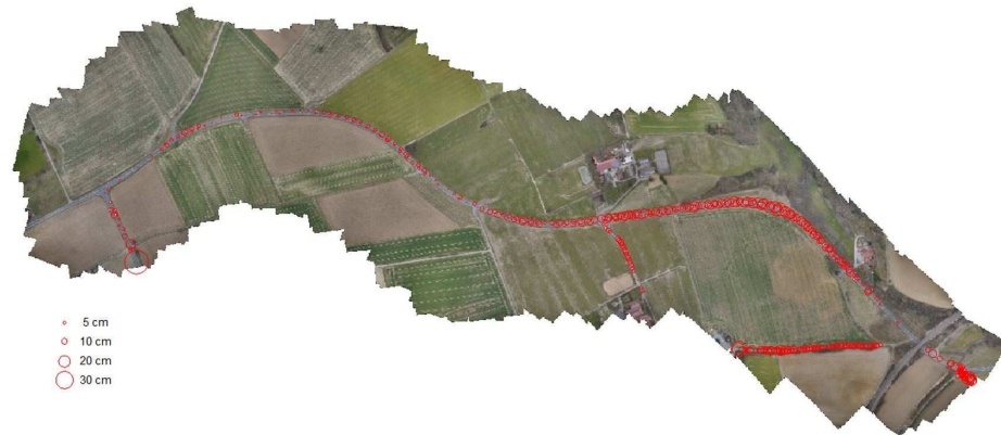
Figure 13: Quality circles depicting the vertical accuracy. The diameter of every circle reflects the quality of height determination (see legend). The reference heights are derived from a kinematic GNSS survey of the road profile.
