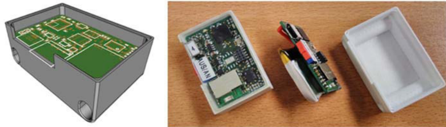
Figure 6: Wearable MEMS inertial sensors with rechargeable battery and Bluetooth module in 3D printed case.
