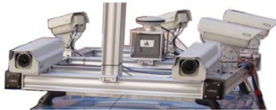
Figure 15: Sensor configuration of the multi-view stereovision IVGI mobile mapping system.
