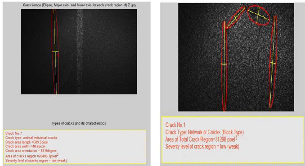
Figure 15: Final resultant images with vertical individual cracks and network of cracks (block type) and their characteristics.
