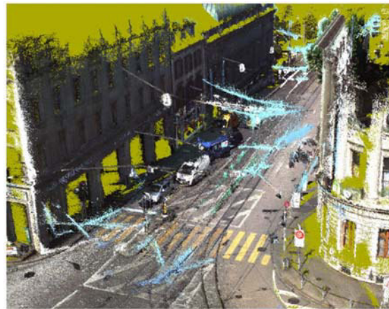
Figure 17: Filtered point cloud generated by incorporating forward stereo imagery and exploiting five match images per base image (c4).
