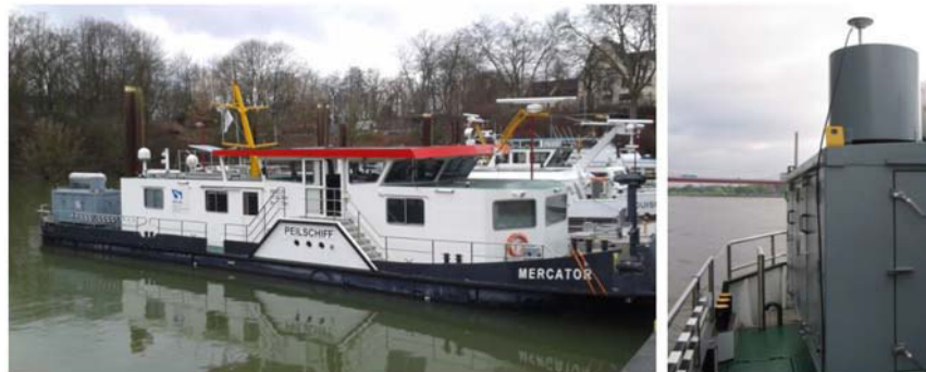
Figure 4: „Mercator“ observation vessel for the measurement data (left figure); GPS antenna over the vessel (right figure).
