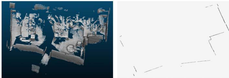
Figure 5: Left: Raw point cloud from Project Tango; Right: Orthographic projected image.
