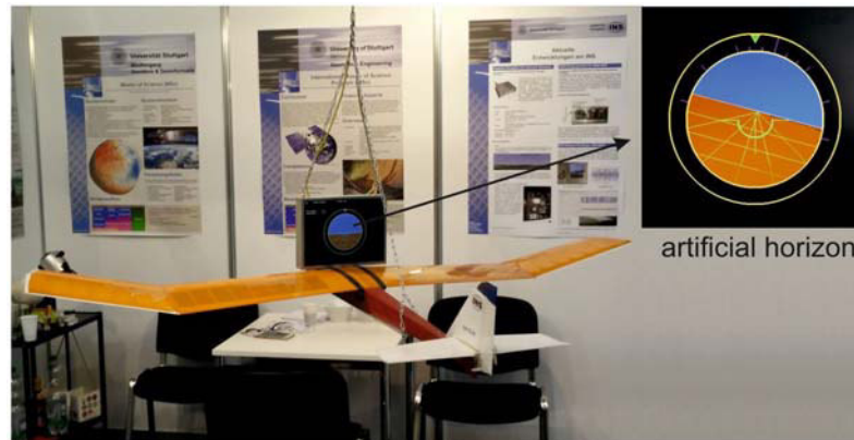
Figure 5: Advanced GPOS-BI mounted on a model airplane.
