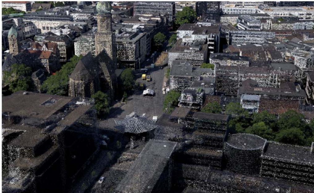
Figure 9: Point cloud from oblique imagery.
