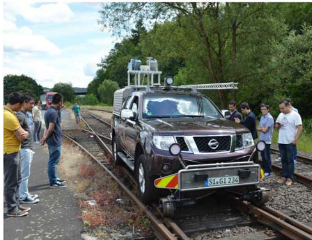
Figure 18: The IGI RailMapper system as during demonstration. The system is installed on a high-rail vehicle - here shortly after railing on the tracks. The measuring sensors are installed in the trunk of the car and lifted up for the survey. The students are waiting to join the test drives.
