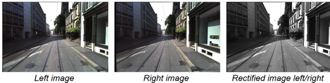
Figure 28: Stereo image pair and rectified image captured by left and right forward looking camera.
