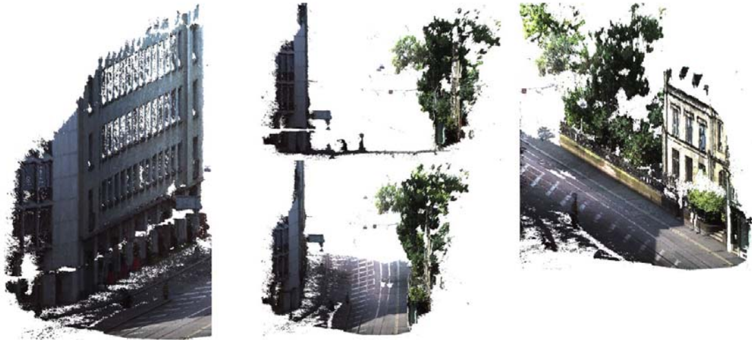
Figure 30: Point cloud generated by SURE from Mobile Mapping Imagery.
