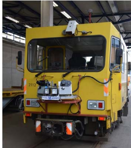
Figure 19: The RailMapper system installed on the SSB vehicle before the measurement campaign (May 16, 2014). The boresight parameters have already been pre-surveyed and the system is now ready to start.
